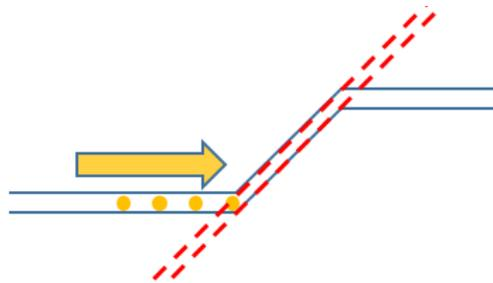
*Figure 4. Proppant screen-out caused by an offset fracture. Hydraulic fracture (solid blue lines) is offset by a natural fracture (dashed red lines). As a result, proppant particles (yellow) cannot enter the narrow inclined portion of the fracture. Yellow arrow indicates the direction of fluid flow and proppant transport.*
