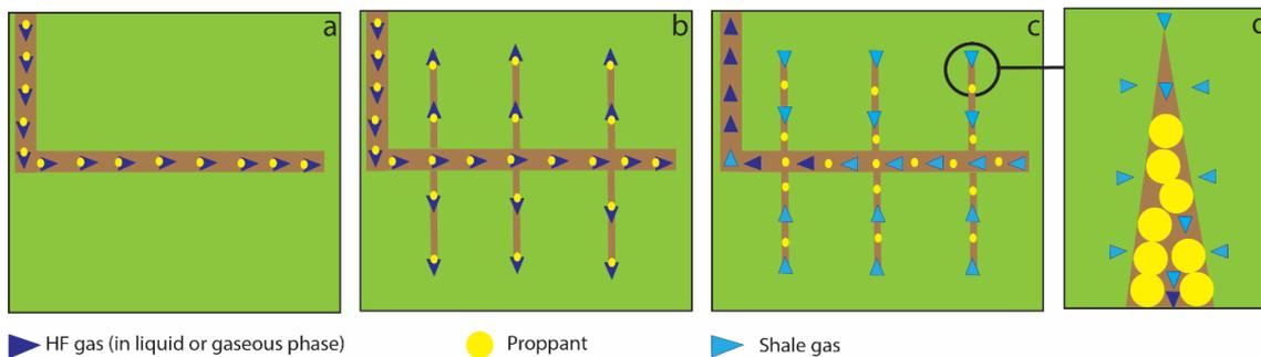
*Figure 5. Hydraulic fracturing using water-free fracturing fluids: The injection of pressurized liquefied HF gas (a) creates fractures (b). Under reduced pressure, liquefied HF gas turns to gaseous form and flows back to the well followed by the shale gas (c). The proppant leaves the fracture opened allowing the shale gas to flow into the well (d).*
