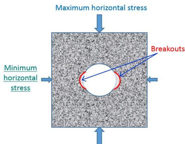
Figure 3. Breakouts around a vertical well.
