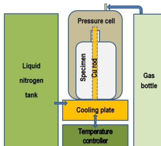
Figure 6. Schematic of an exemplary experimental setup for thermal cycling experiments. Based on (De Andrade et al., 2014).
