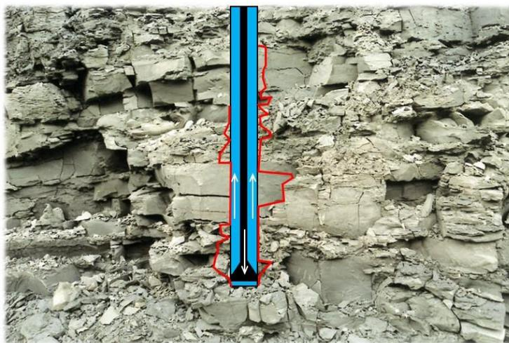
*Figure 2. Fallouts/washouts caused by natural fractures when drilling through a naturally-fractured shale. Fallouts/washouts are delineated with the red line. White arrows indicate flow direction of the drilling fluid in the drillstring (downwards) and in the annulus (upwards). Drillstring is shown in black.*
