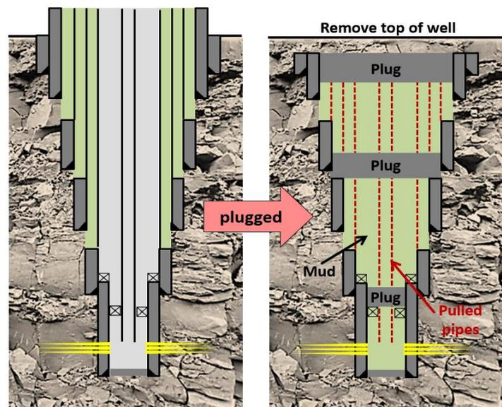
Figure 1. Example of an active (left) and abandoned (right) shale well.
