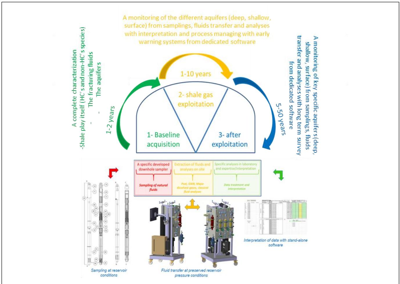
The methodology to deploy in term of geochemistry (with iterative operations) in regard to the shale gas exploitation cycle (baseline – exploitation – after exploitation) for monitoring well leakage.
