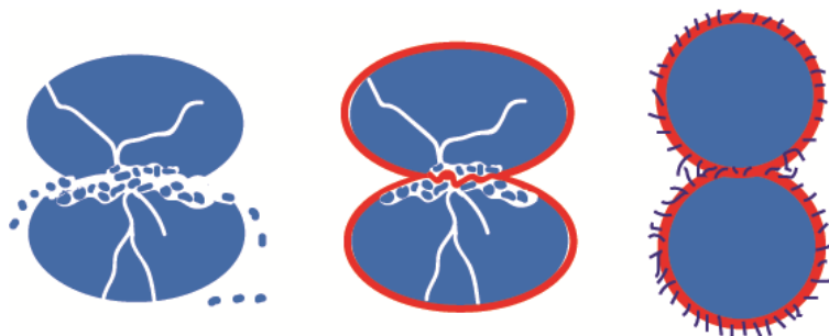
Figure 3. Schematic illustration of proppant particles: Left: no coating – producing fines, Middle: polymer coating – fines migration limited, Right: polymer-fiber composite coating – proppant backflow limited.
